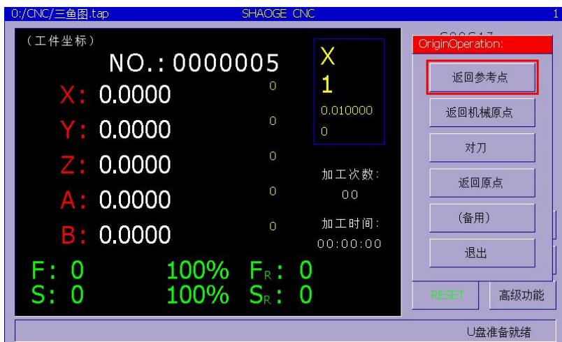
**“Return to reference point”** The Z-axis is raised to the safe altitude, all other axes return to the specified position, and the Z-axis returns to the specified position (this point can be set at the mechanical origin).
