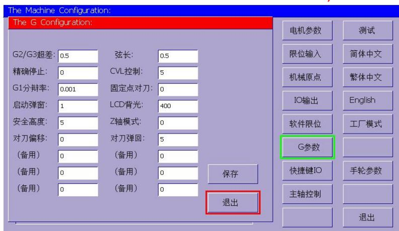
**G2/G3 Tolerance:** Refers to manual calculation or other calculations. G02/G03 is input because of calculation accuracy. The arc center is inconsistent with the given value. At this moment, there is a fault tolerance value, and the system will use the given parameters. , recalculate the ideal center coordinates, detailed description can be seen G02/G03
