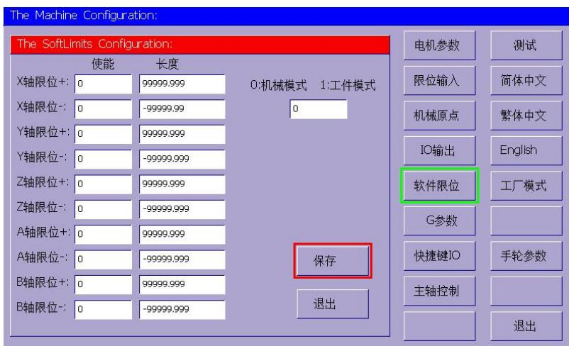
Software limit, generally select the mechanical origin mode, it will decelerate according to the mechanical origin as a reference
