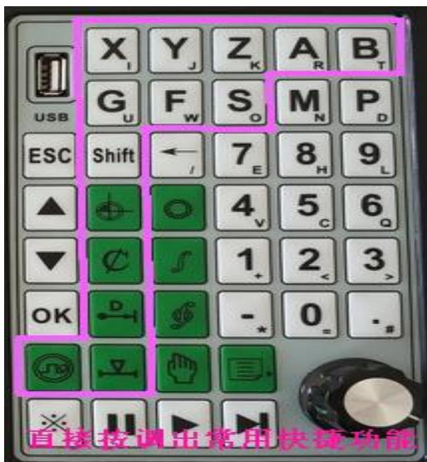
The panel shortcut key X Y Z A B is "direct coordinate operation"
