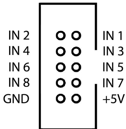
This connector provides input for user-assigned functions.
