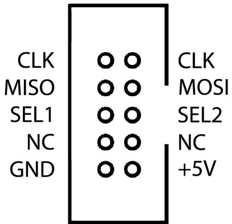
Connector for additional IO extension boards.
