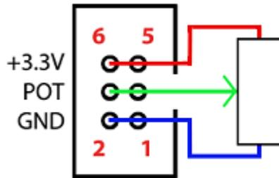
A potentiometer attached to this connector provides a manual jog speed control when using jogging keyboard connected to JOG connector. Mk3 controller also has this pins on jogging connector.
