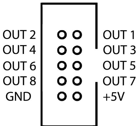
This connector provides 7 digital outputs for control of external devices. The optional 'Output board' links to the Mk3 controller using this connector. Output assignment is controlled in software.
