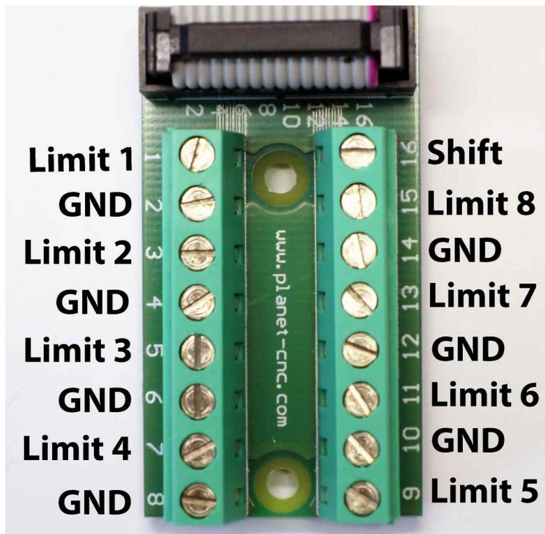
Bellow are wiring plans and pictures that demonstrate wiring of limit switches when 'Normal' or 'Single input' method is used.
