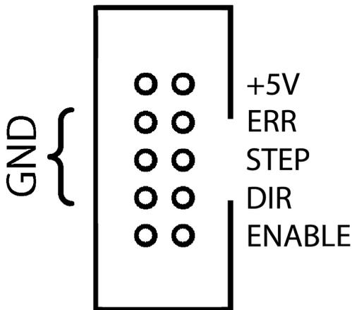
Each connector controls one motor driver. Controller has 9 connectors for axes 1-9. This means 9 axes which can all be moved at same time.
