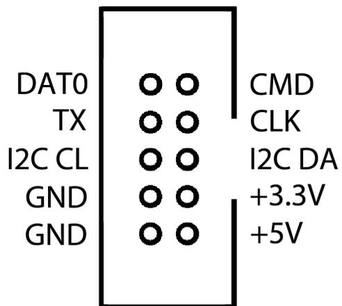
This connector allows use of SD Card with PlanetCNC SD card adapter, I2C and UART protocol devices.
