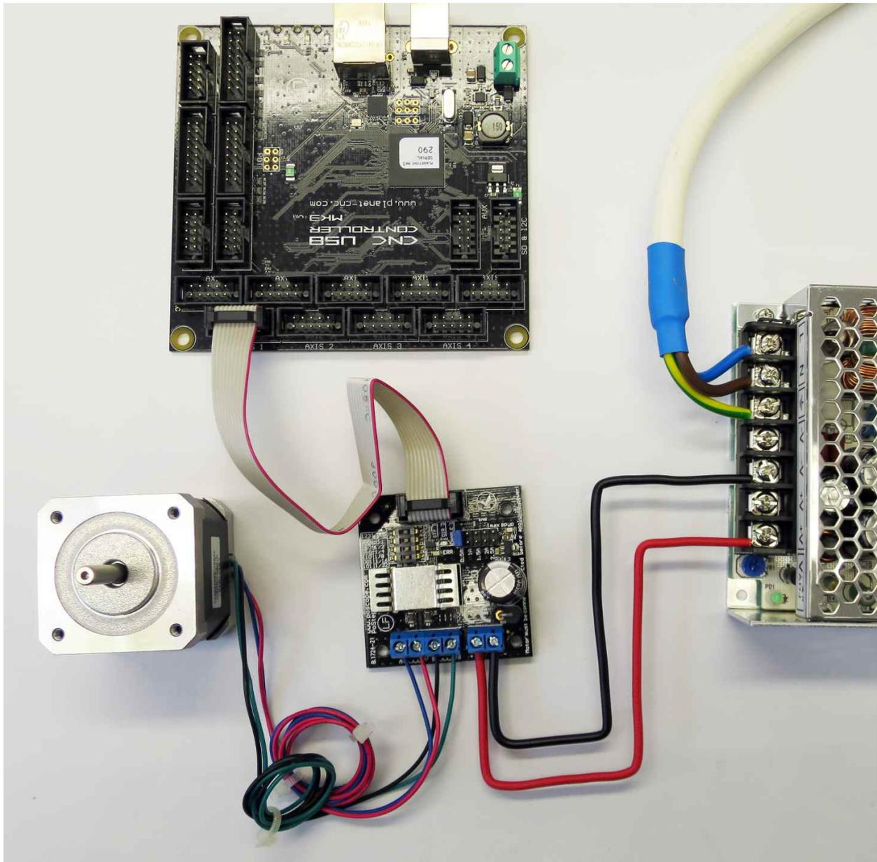
Picture below demonstrates connection of motor driver to Mk2 controller with screw type adapter and connection of controllers external power supply:
