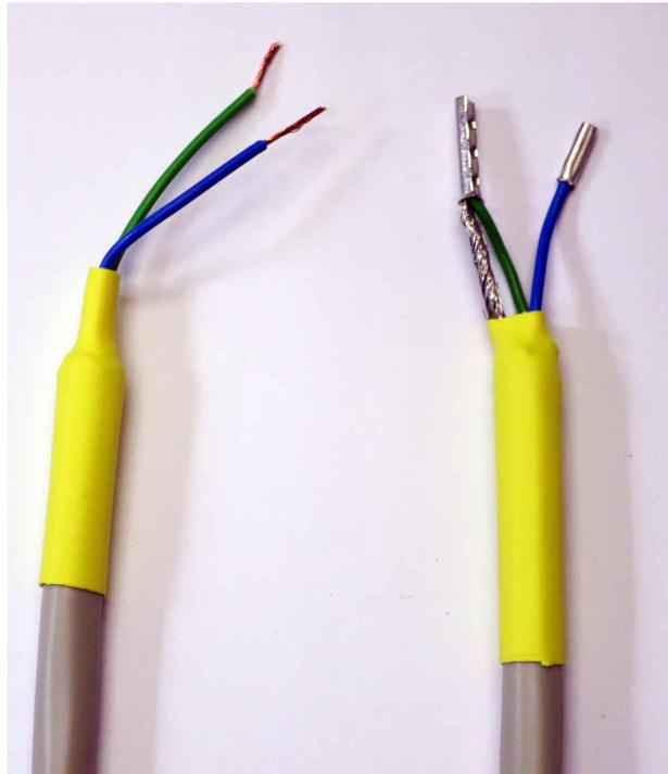
Shield of the cable should be connected to GND only at the end which is connected to controllers input:
