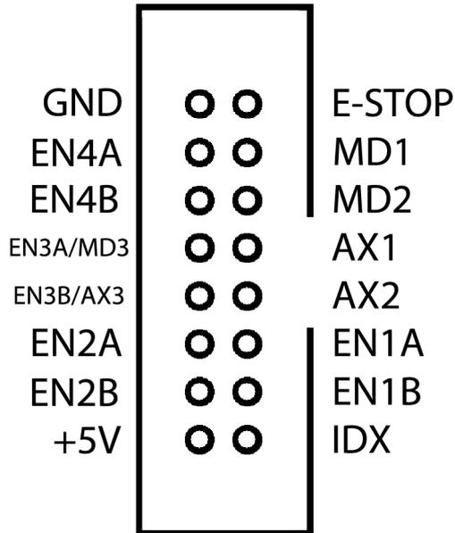
This connector provides inputs for use of MPG pendant devices and E-Stop. Spindle speed encoder for spindle synchronization can also be connected. GND pin provides 'Ground' or common connections.
