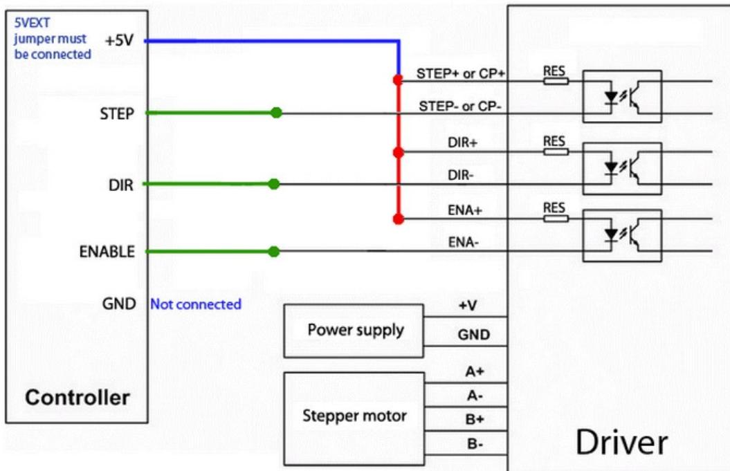
\*STEP input on motor drivers can be also labeled as PUL or CLK.
