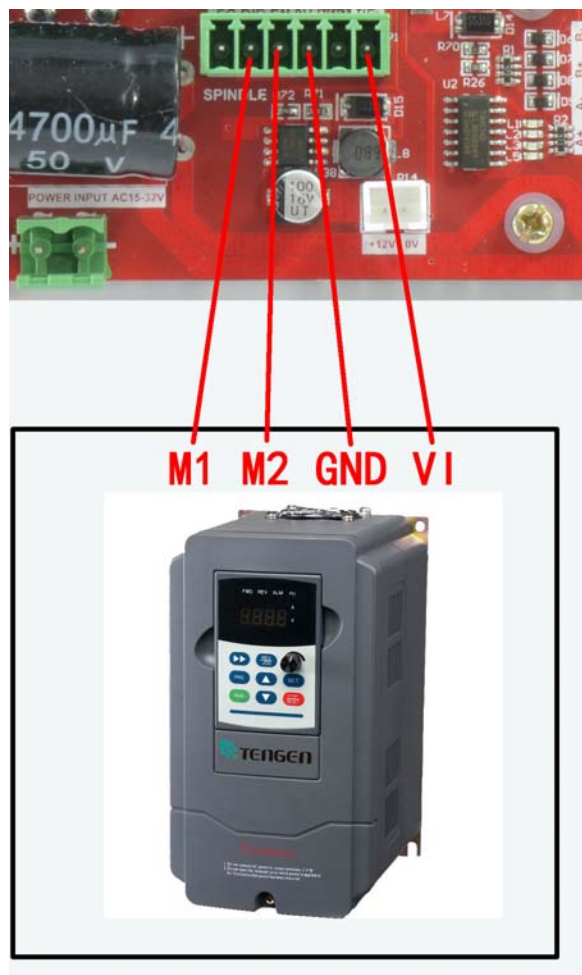
Figure2-4. Wiring with Frequency Converter
