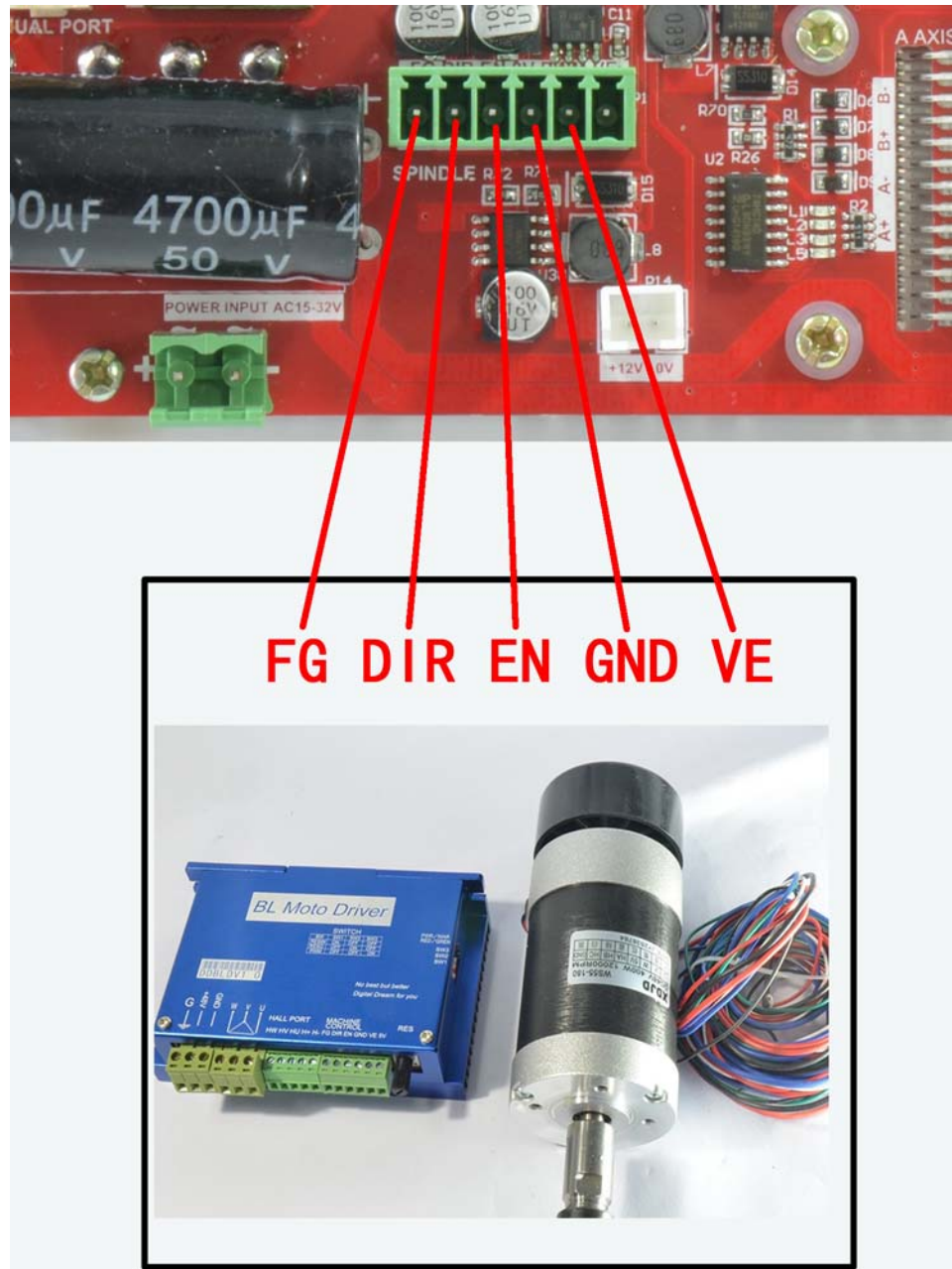
Figure2-5. Wiring with BLDC driver
