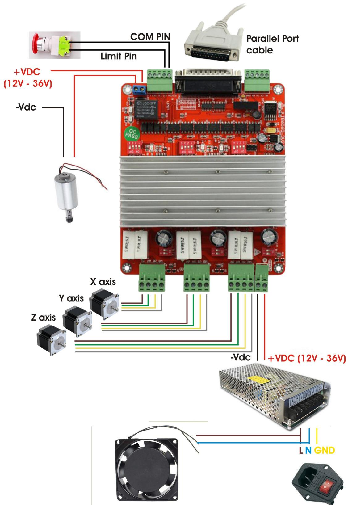
The wirings and connections are shown to the diagram above. The Spindle is not included to the kit.
