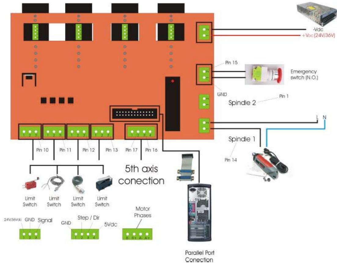
Parallel port pins for Step and Direction:
