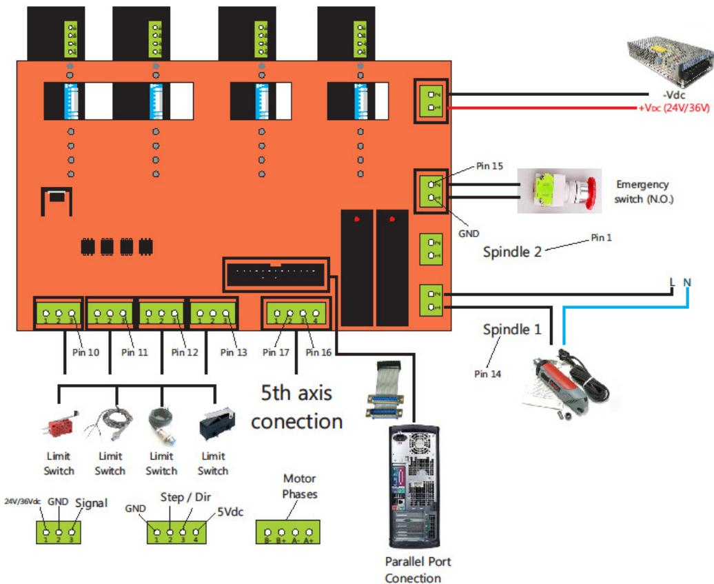
Parallel port pins for Step and Direction:
