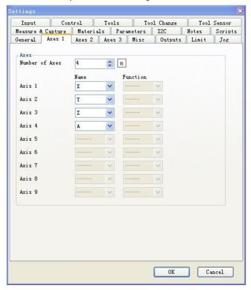
number of axes to choose the count of axes, following R button is to set Define name for each axes.
