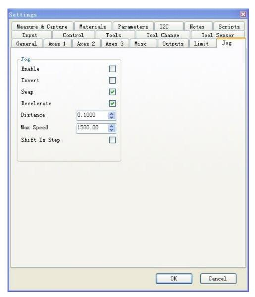
Enable is needed if you want to connect a manual device, here we choose yes. Invert is electric level invert, to fit our device, don't choose this one.
