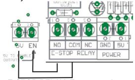
Basic connection of the E-STOP RELAY. For more advanced connections check: <u>http://cnc4pc.com/Tech\_Docs/E-STOP\_RELAY.pdf</u>
