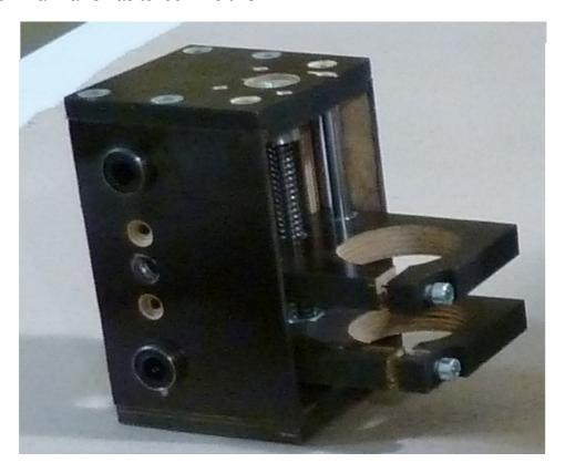
Next you have to assemble the main body of the E-Graver. Look carefully the next photo. The parts with the linear bearings have the trapezoidal nut. This nuts are asymmetrical. It means that the one side has bigger distance than the other. You have to put the parts as the photo below shows:
