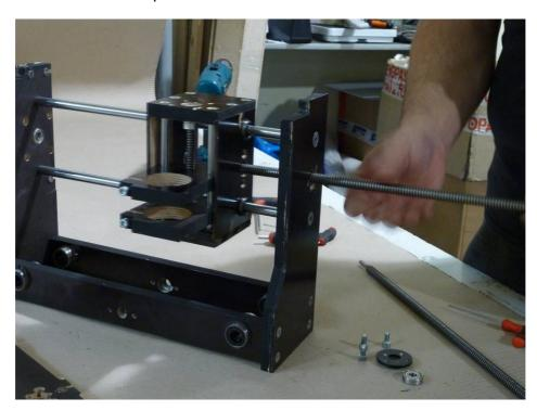
The trapezoidal lead screw locks into with a 608zz Double Shielded Ball Bearing 8x22x7mm and a Bearing adjustment flange.
