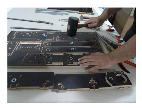
The picture below shows you the 28pcs Allen screw nut 6mm installation:
