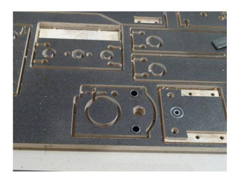
Now you have to set up the linear motion bearings .Remove the wood from the sockets of the bearings and with a rasp remove the remaining tabs.
