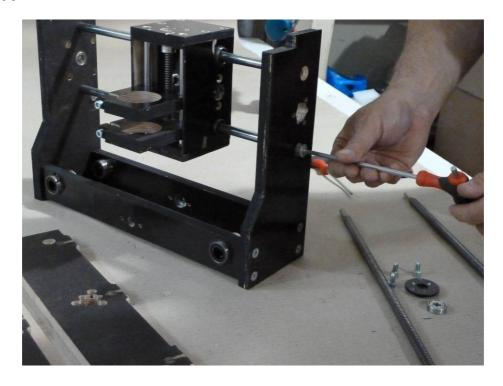
It's time to screw the trapezoidal lead screw shaft of Y axis.
