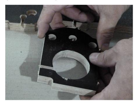
You have to use a drill driver and a drill with diameter 6mm and make a drill hole as you see:
