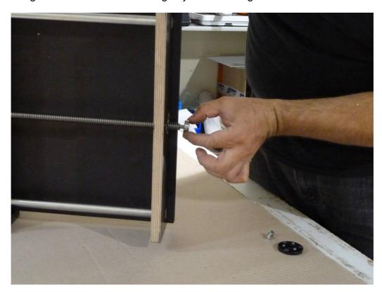
Adjust the X axis metal flange with the same way as you do with the Y axis metal flange.
