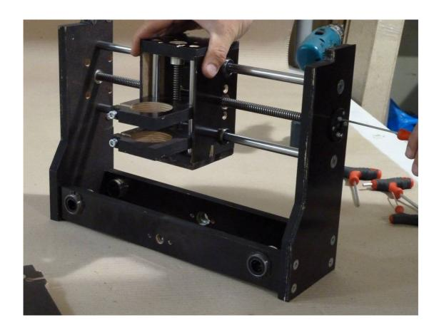
You have to assemble now the front and back of the kit. The parts that you need are 2 pieces of linear motion slide shaft D16mm, allen flat head screw 8mm X 25mm, and the front and back of the wooden parts.
