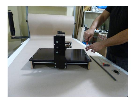
Screw the trapezoidal lead screw shaft of X axis.
