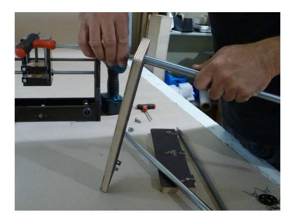
Get the part that fits on the stepper motor and make it the back part of the kit. The part that fits on the metal flange make it the front part.
