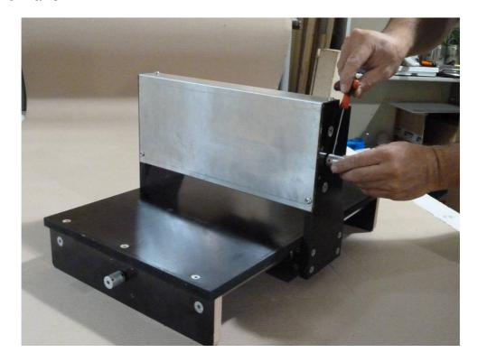
Your Kit is almost done! The two motor mounts that include into the pack will be install on to the machine when you decide to assemble the **electronic** parts of the Kit!
