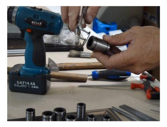
When you finish with seeger installation you have to put the linear motion bearings on their position. You have to take care with the way that linear motion bearings will set up. The side with the seeger must be at the bottom of
