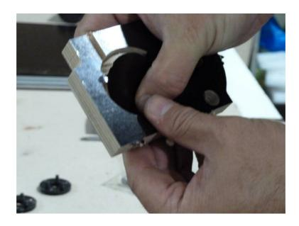
With a round rasp or sandpaper remove and the inner wood that is hold with the inner tabs:
