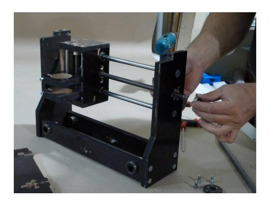
Allen Head screw 6mm X 16mm holds the flange from the inside.
