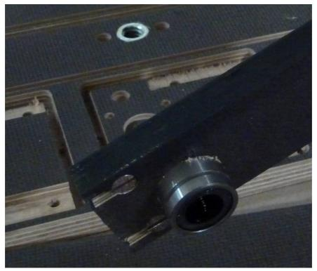
Install with this way all the linear bearings. The side without seeger has to be at the same side with the Allen screw nut.
