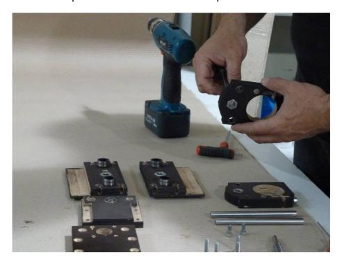
A few turns later screw the second part. The distance between them depends on the basic body of the spindle.
