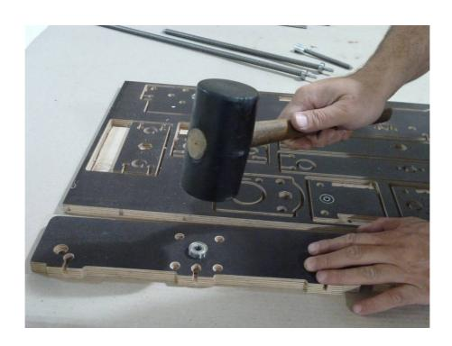
$\label{eq:filling} \mbox{Fill in the Hexagon trapezoidal nuts 12mm also with the same way .}$  With a plier remove the rubbish wood that is holded with the tabs
