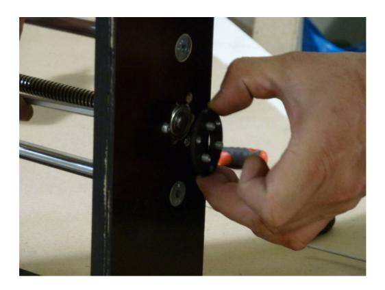
Three no head allen screws on the flange, regulate the 608zz Double Shielded Ball Bearing.
