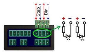
Step / dir signal inputs of the motherboard are made with the use of optical-insulation 5V technology, as in most motor controllers, therefore these inputs are connected in the same way "instead of" the stepper motor controller.
