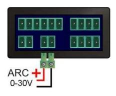
The controller has a configurable voltage plasma arc measurement input. To the input you can connect voltage from the 1/20 or 1/50 voltage divider. The input is completely galvanically separated and does not require additional separation. The selection of division is carried out by appropriate setting in the controller service menu.
