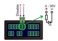
The Disable input is designed to stop the work of THC by program which allows using the Anti-dive feature or turning on THC after measuring the penetration time by the program which frees the user from setting the Delay-Time in the THC menu.
