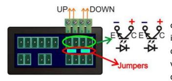
The UP / DOWN outputs are OC optically insulated outputs (open collector). The maximum voltage that can be connected to the UP /
