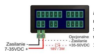
To supply power to the controller, use an AC adapter with voltage of 7-35V / 150mA min. Voltage stabilization is not required. The system can be powered from a power supply with a higher voltage (35 - 50V) – then use 18V / 3W Zener diode.
