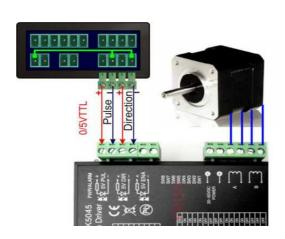
allows control of optical insulation input LEDs used in most controllers. The output signals "-" are connected inside the controller to the terminal "-" of the power supply, as indicated with the green line in the picture.
